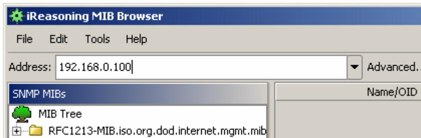
In the **address** field enter IP address of IP Watchdog and press **Advanced**
