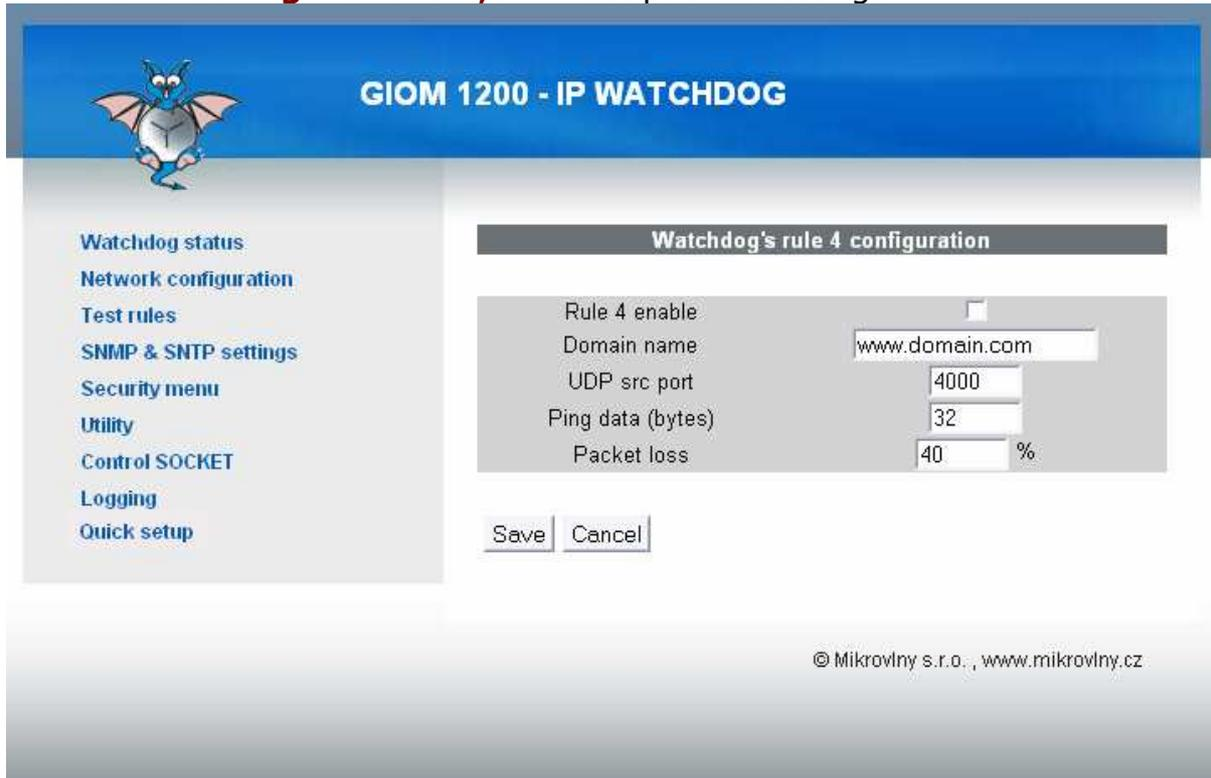
The screenshot shows the 'GIOM 1200 - IP WATCHDOG' configuration interface. On the left is a navigation menu with options: Watchdog status, Network configuration, Test rules, SNMP & Sntp settings, Security menu, Utility, Control SOCKET, Logging, and Quick setup. The main content area is titled 'Watchdog's rule 4 configuration' and contains the following settings:
