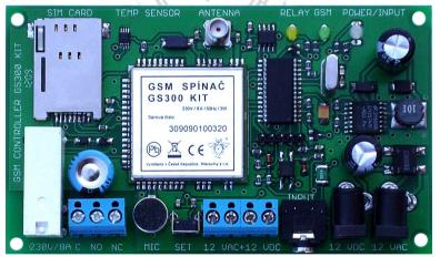
SIM CARD-SM CAR slot, **TEMP SENZOR**-Ten perature sensor ANTENNA- Connector SM Af for connecting any external G SM antennas. RELAY/GSM/POWER/INPUT-LD indicators.
